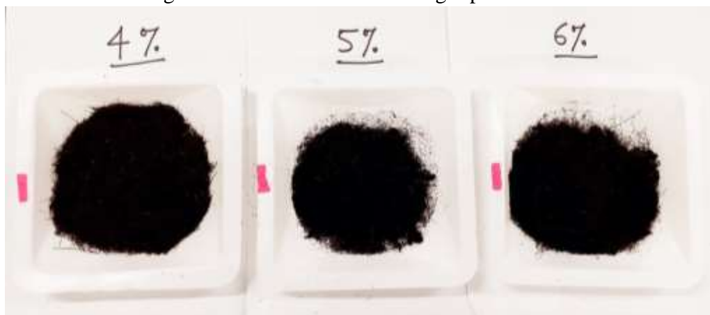
Figure 2 Treated SPFs in 4%, 5% and 6 % w/v alkaline solution
