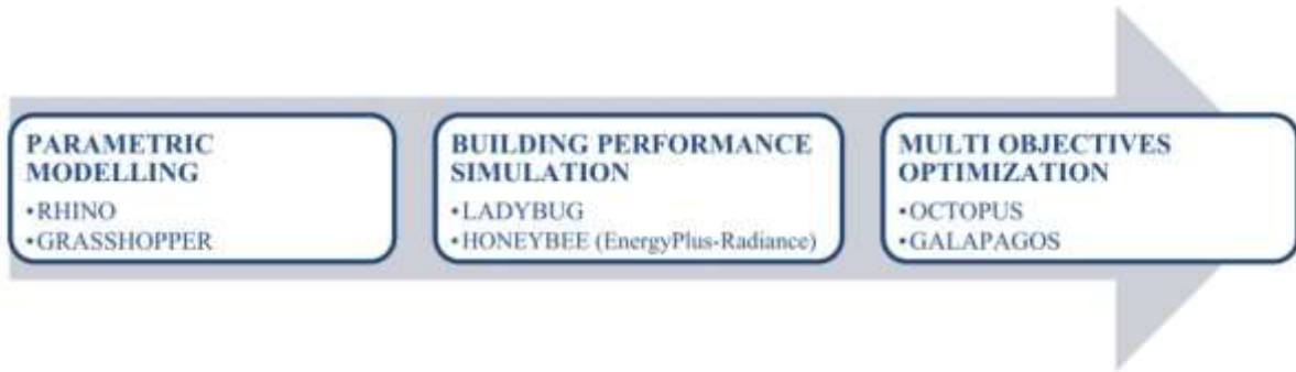
Figure 3. A suggested workflow for parametric based optimization in Grasshopper (Toutou et al.,2018)
