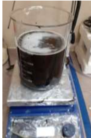
Figure 1 Alkaline treatment of sugar palm fibers
