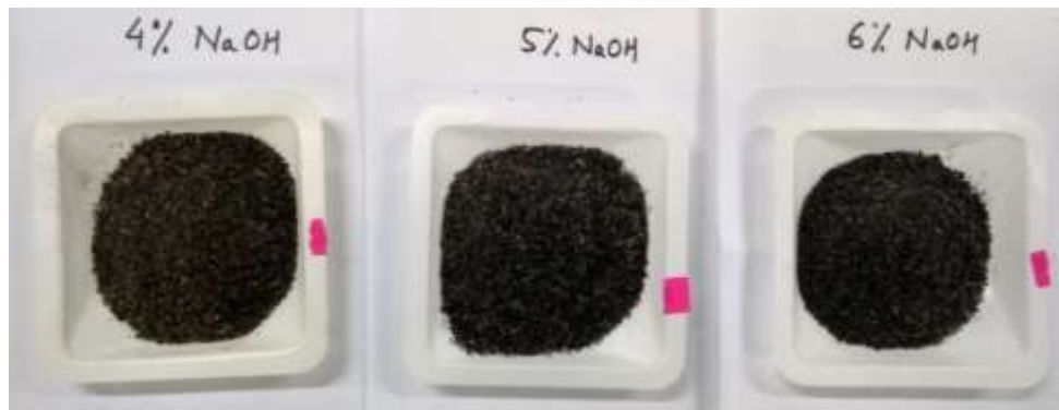
Figure 3 Alkaline treatments (at 4, 5, and 6%) SPF mixed with PLA
