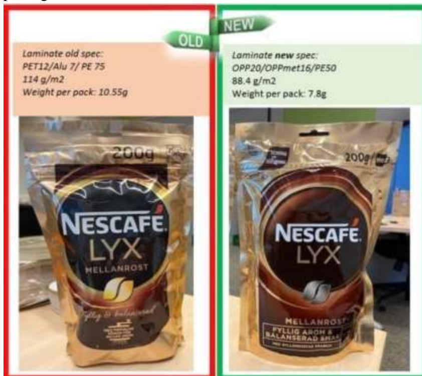
Fig.4. Comparison of the old structure and monomaterial structure of Nescafé doypack packages
